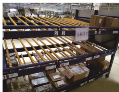
Flow roller rails in express company
