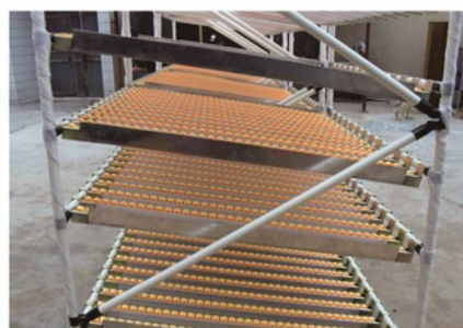
Flow roller rails on lean pipe rack
