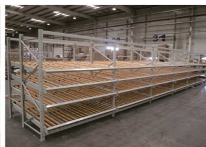
Flow roller rails in distribution center
