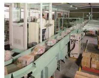
32. Package distribution line on belt conveyors
