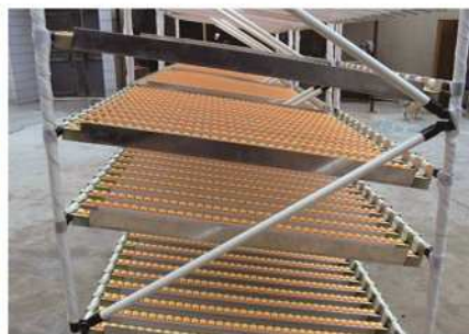
Flow roller rails on lean pipe rack
