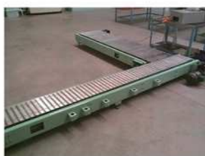
Slat chain conveyor connection
