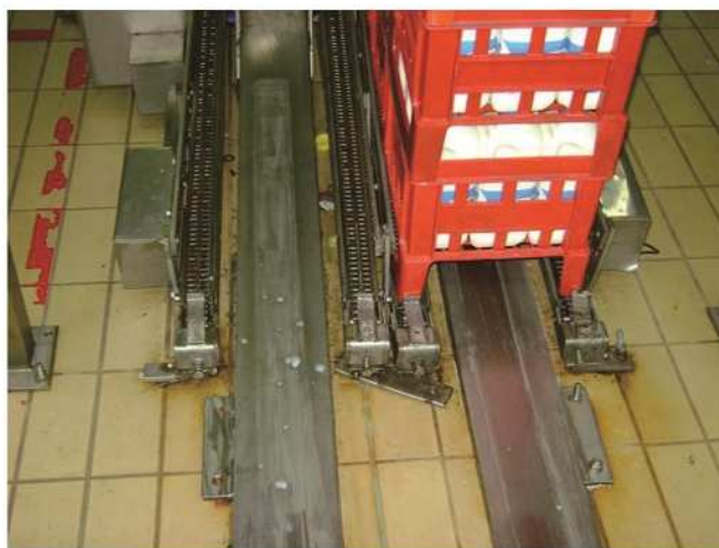
Full stainless steel application with turnover boxes directly on the conveyor
