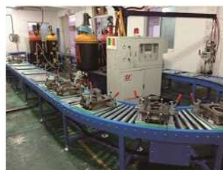
Endless roller conveyor for molds assembly
