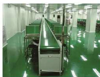
3. Belt assembly line with working stations
