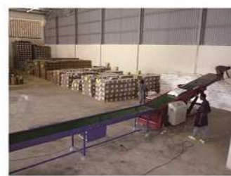
36. Offload stacked bags and load to a container
