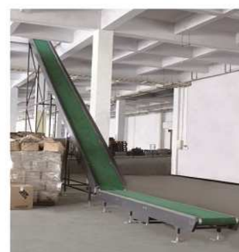
Inclined belt conveyor between floors
