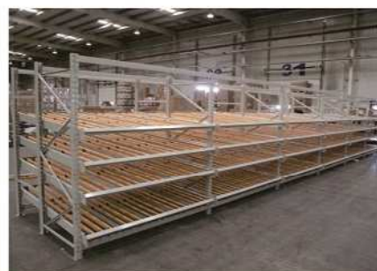
Flow roller rails in distribution center
