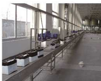
26. Storage battery unit delivery line
