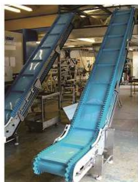
Inclined cleated belt conveyor
