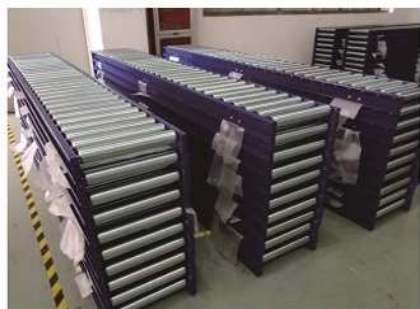
3M gravity roller conveyor bodies
