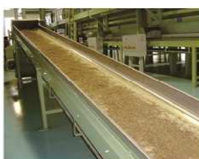
Inclined conveyor for tobacco
