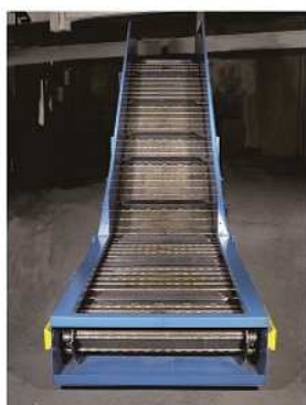
Inclined conveyor with steel slats
