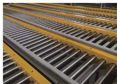
Optional chain cover protection design for extra safety
