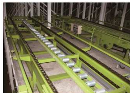
Double chain track with middle gravity rollers
