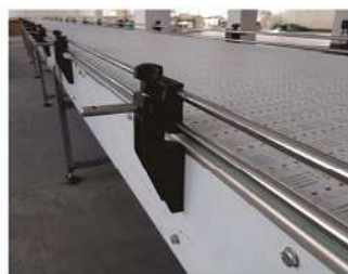
Side guide available and as width control
