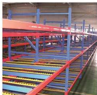
Racks with flow rails
