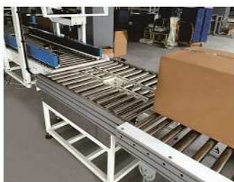
29. Roller conveyor in packing system
