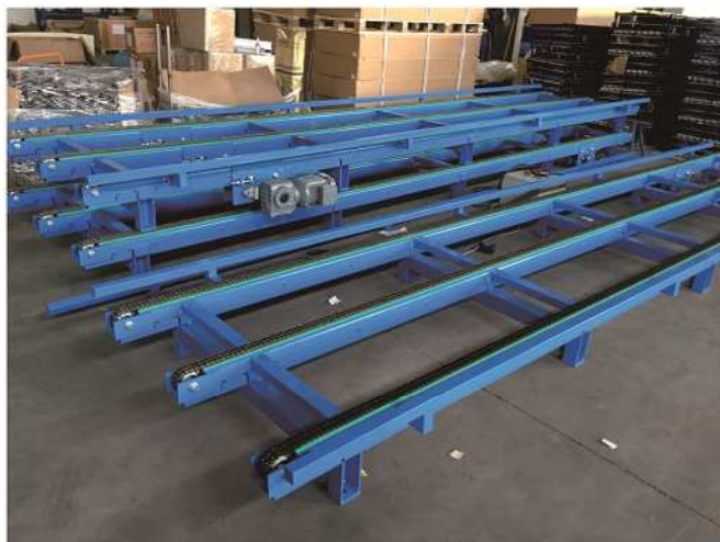
Three-Chain-Track pallet conveyor, ground type with height as low as possible
