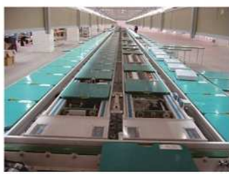
14. Differential chain storage line
