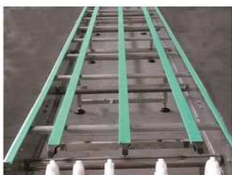
Wear-proof guide bar beneath modules
