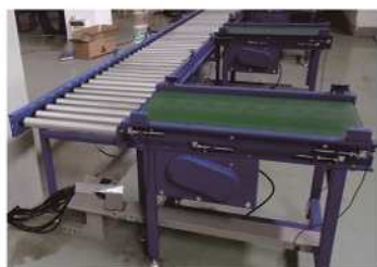
Roller conveyor and belt conveyor combination
