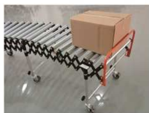
End stopper to avoid packages falling down
