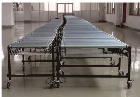
Different conveyor width possible, max. 1000mm
