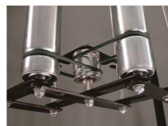
Less noise with O-belt driving
