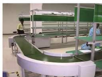
7. Endless belt conveyor assembly line
