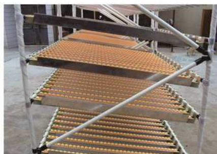
Flow roller rails on lean pipe rack
