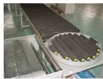
15. Gravity rubber coated roller turn table
