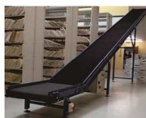
Inclined conveyor in storehouse
