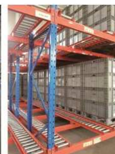
Flow rails of steel rollers
