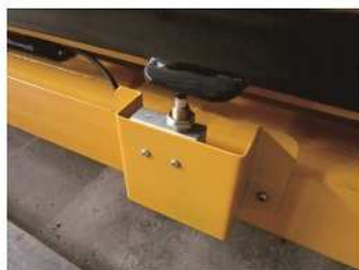
Safety protection: range limit switch
