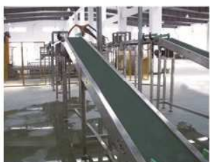
Inclined conveyor in steel steel frames
