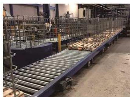
Roller type is also popular especially in accumulation.
