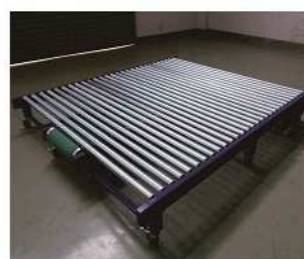
12. Belt driven idle roller conveyor
