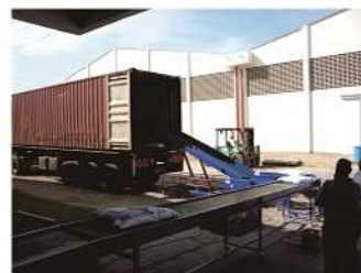
34. Loading soft woven bags from storehouses
