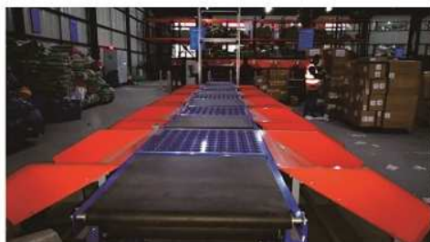
90 Deg. double side sorting diverter
