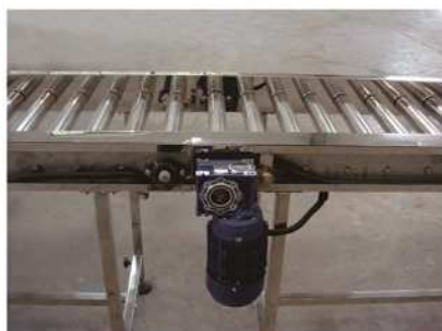
Optional conveyor motor unit: worm gear motor type
