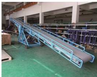
2. Two-wing multi-height loading conveyor
