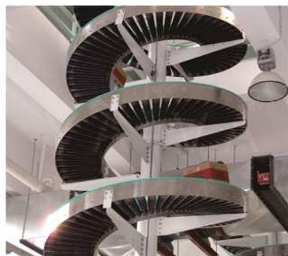
Roller option: straight or coned; plastic or steel
