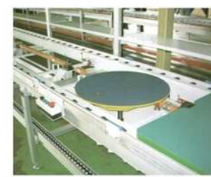
16. Assembly line with swivel turning table
