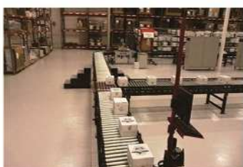
11. Cartons distribution with roller conveyors
