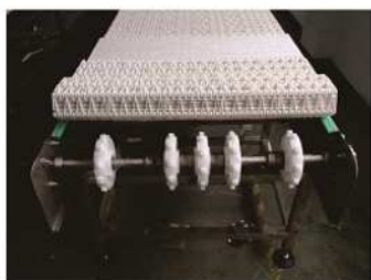
Driven by Low noise PP material sprocket
