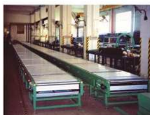
Linear heavy duty slat chain conveyor
