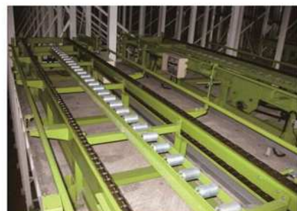
Double chain track with middle gravity rollers
