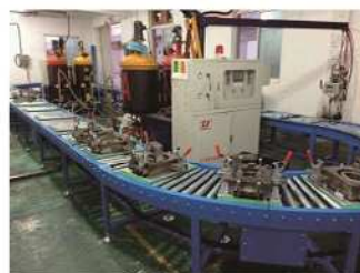
Endless roller conveyor for molds assembly
