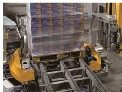
Pallet conveyor combined with film packing machine
