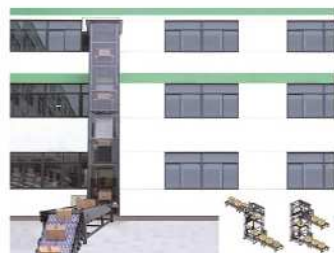
5. Z typed vertical conveyor outdoors
