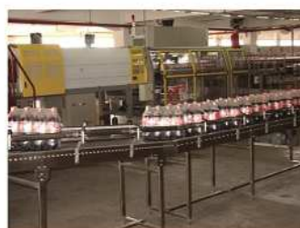
5. Coke package delivery line after shrinking
