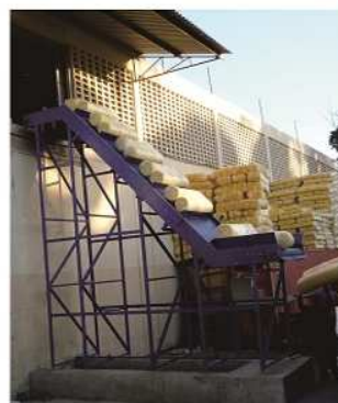
Inclined cleated plastic modular conveyor
