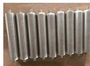
Roller with pinned hexagonal shaft
