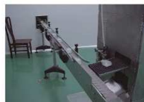
Slat C/V connecting to other equipment
