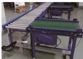
Roller conveyor and belt conveyor combination
