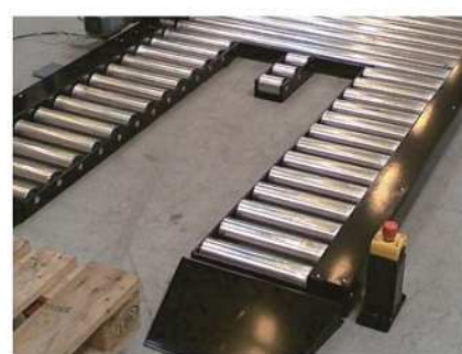
Pallet roller conveyor end section for pallet removal
