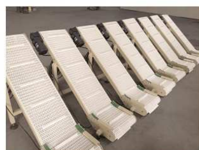
Mini light-duty cleated modular conveyor
