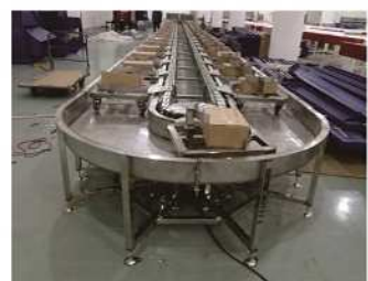
13. Endless chain truck conveyor for cooling
