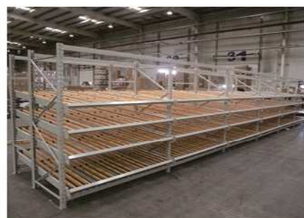
Flow roller rails in distribution center
