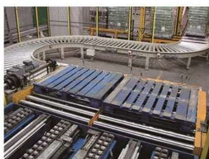
Pallet roller conveyor can be flexible in layout.
