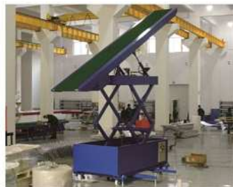
1. Hydraulic lifting inclined conveyor
