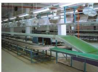
6. Belt conveyor production line
