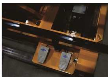
Optional pedal control for lifting and lowering
