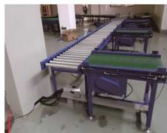
25. Interflow line with belt and roller c/v
