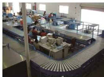
33. Package distribution line with roller conveyors
