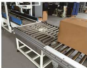
29. Roller conveyor in packing system
