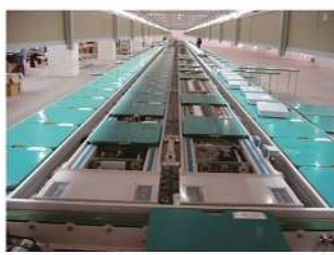
14. Differential chain storage line
