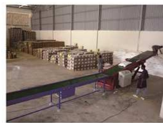
36. Offload stacked bags and load to a container
