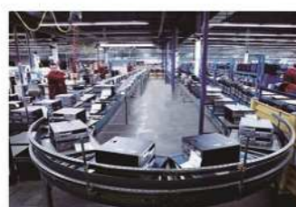
11. Pallet assembly line on roller conveyors
