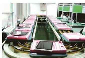
10. Endless pallet assembly line with tracks
