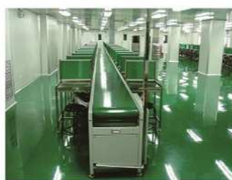
3. Belt assembly line with working stations
