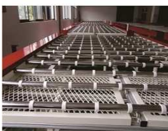
11. Roller with teflon as laminater outlet conveyor
