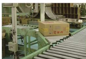
15. Cases interflow roller conveyor section
